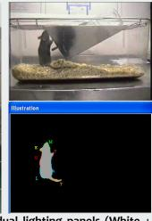
The IVC-RackScan Rack comes fitted with dual lighting panels (White + IR light) for continuous automated 24-hr analysis, and associated filters, isolation and air circulation required from an IVC system. The included cameras auto-switch between day mode and night mode, hence, no user intervention is required.
